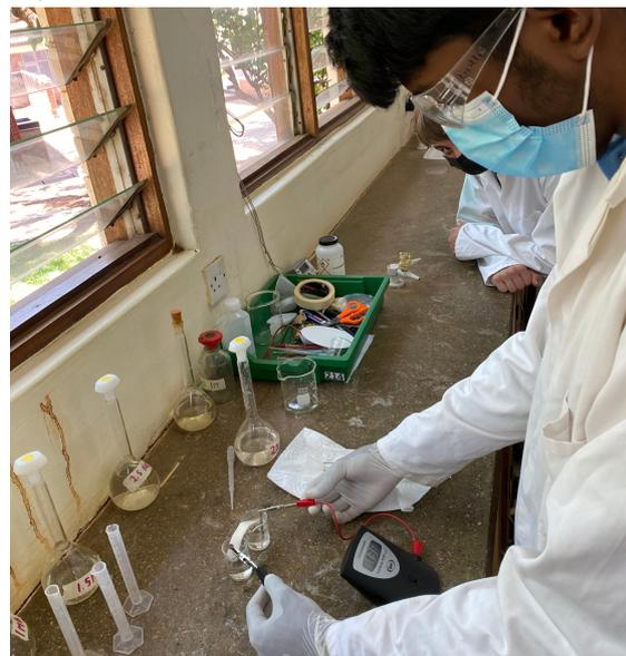
For my IA I am looking at Voltaic Cells and how the concentration of a solution affects the voltage output. I am trying to create a battery using iron and magnesium to investigate if they are a better option for batteries in the future. Aditya Chockalingam
